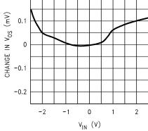
**Typical Performance Characteristics**  $V_s = +5V$ , Single Supply,  $T_A = 25^{\circ}C$  unless otherwise specified (Continued)
