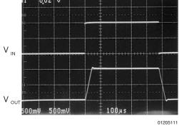
FIGURE 7. Pulse Response of LMC6462 Circuit in *Figure 6*
