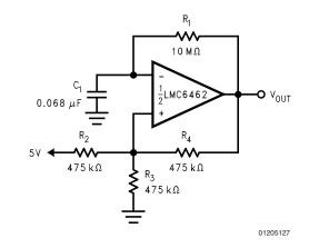
FIGURE 21. 1 Hz Square-Wave Oscillator
