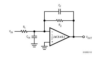
FIGURE 8. Canceling the Effect of Input Capacitance
